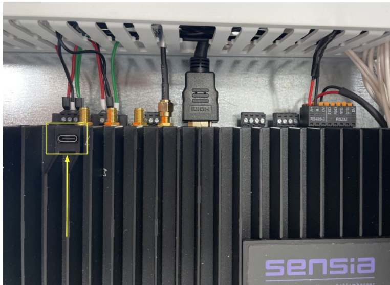
Figure 5.1—HCC2 USB-C connector for laptop connection
