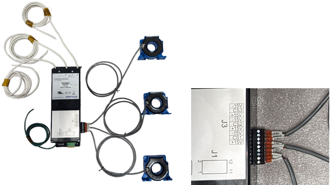
Figure 4.10—Current sensor to PowerDAQ (J3) connection
